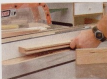
Plunge cut the hutch door stiles
