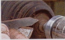
Cut a spigot for the base
