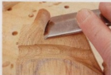
Round side of head (#5 gouge, face-down)
