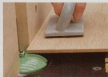
Rout the center raised panel
