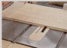
Cut a dado in the center of the bottom shelf
