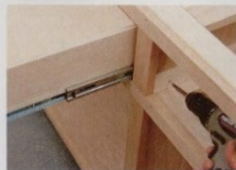
Install cleats for drawer slides
