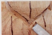
Round away from centerline to junction (#2 gouge)
