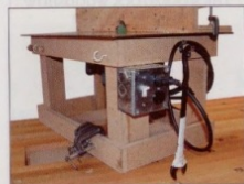
Switch to turn on router and vac simultaneously
