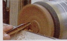
Cut bottom slightly concave
