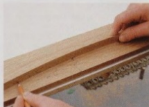
Draw the arc on the bottom rail
