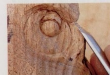
Round top of whiskers (#2 gouge face-down)
