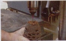
Drill the insert holes
